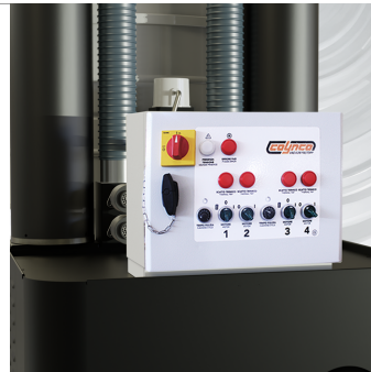
SAFETY Control panel Turbines and cleaning system
